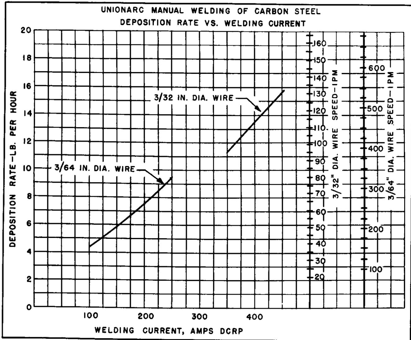
FIG. 2 - Deposition Rates for UNIONARC Welding Process
